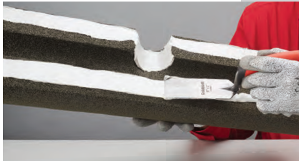
Spreading of joint sealants to full-depth
